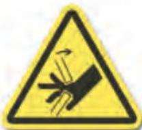
Be careful! Fingers or other body parts of a user and/or assistant can be trapped between the device's parts during folding, unfolding or adjusting of the device. Be extremely careful when adjusting the device. Observe the dimensions of gaps between the device's parts to avoid trapping your fingers or other body parts.
